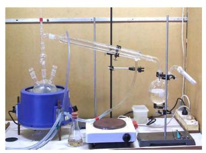
Fig 20.5: Glass distillation system
